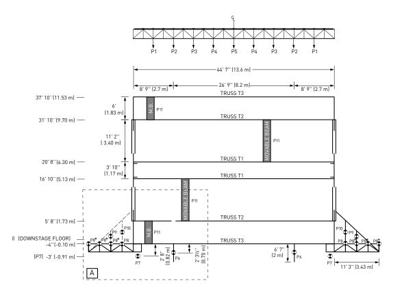
MAXIMUM LOAD BEARING CAPACITY: 47000 lbs (21319 kg)\*
