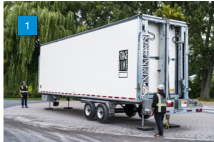
Position and level the trailer. Lower gooseneck.
