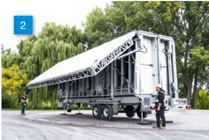
Hydraulically deploy the floor and roof panels.
