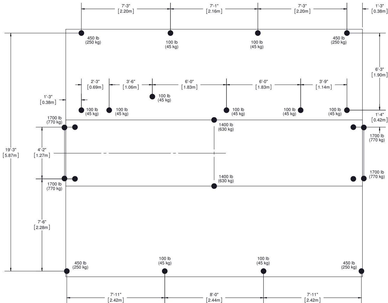
● FLOOR STABILIZERS, EXTENSIONS AND LEVELLING JACKS
