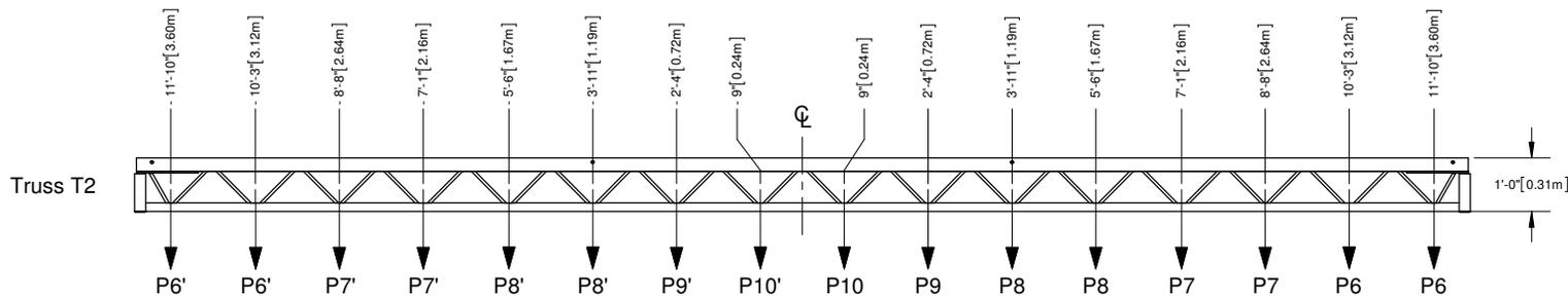
$$\text{Truss T2**}: \frac{\text{Load P6}}{\text{Capacity P6}} + \frac{\text{Load P7}}{\text{Capacity P7}} + \frac{\text{Load P8}}{\text{Capacity P8}} + \frac{\text{Load P9}}{\text{Capacity P9}} + \frac{\text{Load P10}}{\text{Capacity P10}} \leq 1.00$$
