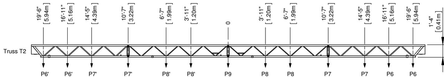
$$\text{Truss T2}^{**}: \frac{\text{Load P6}}{\text{Capacity P6}} + \frac{\text{Load P7}}{\text{Capacity P7}} + \frac{\text{Load P8}}{\text{Capacity P8}} + \frac{\text{Load P9}}{\text{Capacity P9}} \leq 1.00$$
