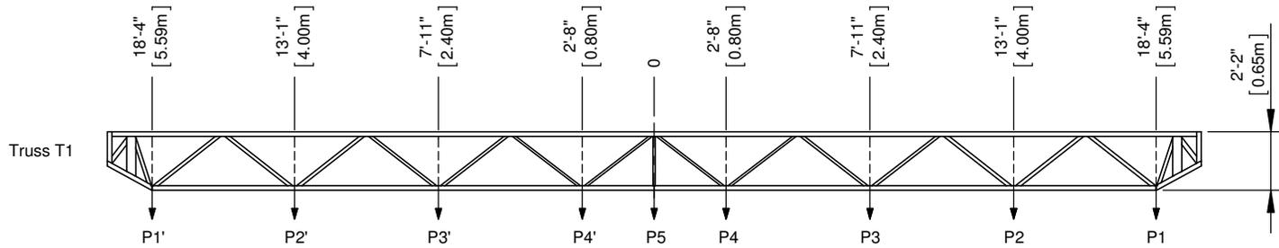
$$\text{Truss T1}^{**}: \frac{\text{Load P1}}{\text{Capacity P1}} + \frac{\text{Load P2}}{\text{Capacity P2}} + \frac{\text{Load P3}}{\text{Capacity P3}} + \frac{\text{Load P4}}{\text{Capacity P4}} + \frac{\text{Load P5}}{\text{Capacity P5}} \leq 1.00$$
