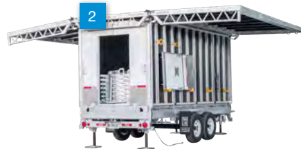
Trailer sides and floor panels equipped with gas springs. Easily deployed manually.
